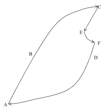
The half-cycle ABC is that without creep, which would be constructed using the unmodified Ramberg-Osgood equation. The half-cycle CEFDA is that with creep and would be constructed using the modified Ramberg-Osgood curve. The difference from the treatment of Figure 1, though, is that in constructing CEFDA the adjusted stress range is not equ.(10) but,
