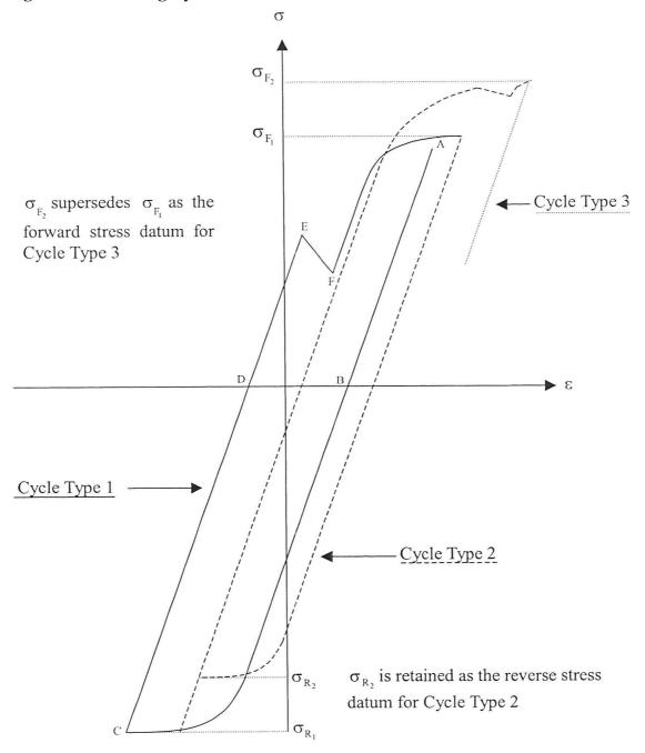
Similarly, cycle type 3 is evaluated in the same way and positioned along the stress axis so that its forward stress datum equals that from the previously established cycle type 2, i.e.,  $\sigma_{F2}$ , as shown above.
