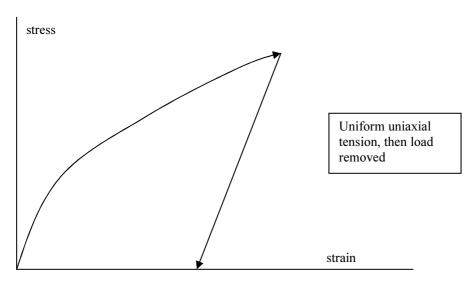
But note that we end up with zero stress only because the uniaxial specimen was assumed to be uniformly stressed. So, a return to zero load means a return to zero stress.
