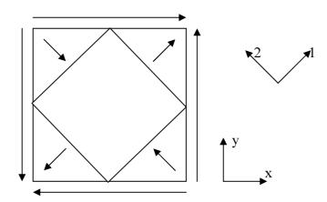
The resolved force on each small triangle is  $2 \times (\tau/2) \times (1/\sqrt{2}) = \tau/\sqrt{2}$ . But the length of the side of the smaller, rotated, square is only  $1/\sqrt{2}$ , so the direct stresses are just equal to  $\tau$  in magnitude, one tensile and one compressive, as illustrated.
