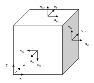
Note the directions of  $\sigma_{zx}$  and  $\sigma_{zy}$ , as a result of the front face of the cube having its normal in the negative z-direction.
