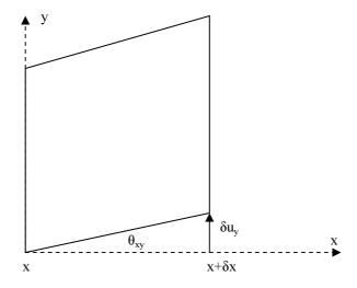
When the distortion is of this form, the engineering strain,  $\gamma_{xy}$ , is equal to the angle by which the element of material is distorted by shear,  $\theta_{xy}$  (for small angles so that
