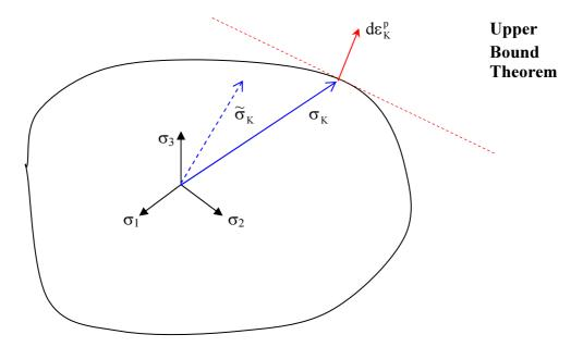
The stress with the tilda is the true collapse stress;
