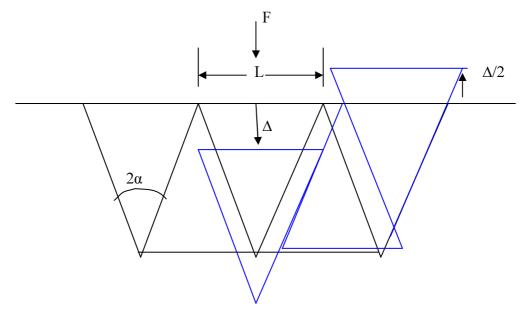
The blue lines show the displaced triangles – on one side only – due to a downwards displacement of the indenter by  $\Delta$ . (Apologies for the distortions – my skill with WordArt is poor).
