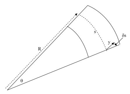
The bending strain at a distance y from the neural axis is  $\varepsilon = \frac{\delta s}{s}$ .
