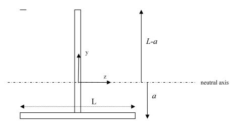
Both legs are of length L and thickness t, and for simplicity we shall work in the approximation  $t \le L$ . We wish to find the position, a, of the neutral axis above the bottom leg. The contribution to  $\int y dA$  of the bottom leg is approximately -aLt,
