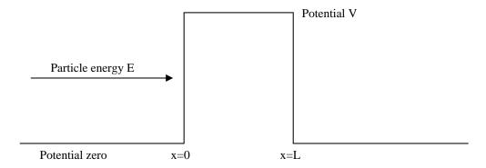
In classical physics, a particle with energy, E, less than the height, V, of the potential barrier has no chance at all of penetrating the barrier. But in quantum mechanics, there is a chance that it will. The probability that a particle penetrates the barrier reduces as either height, V, or the width, L, of the barrier increases. In this note, the fraction of incident particles penetrating the barrier is calculated using the appropriate solutions of the Schrodinger equation.
