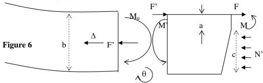
In the above Figure we have used the Bueckner equivalent loading. Thus, the uncracked stress N/b has been applied to the crack face. Hence, the load on the crack face is N' = (c/b)N. This is equilibrated by the sum of the reaction loads on the ligament, F, and at the junction with the bulk of the cylinder, F'. Hence,
