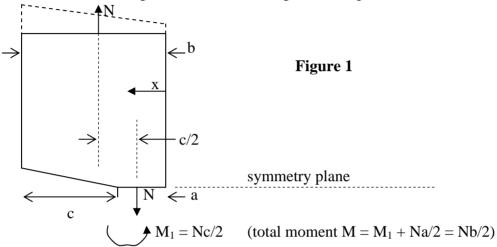
The moment  $M_1 = Nc/2$  is required for equilibrium. Its sense would cause the ligament to rotate anti-clockwise with respect to the end of the plate. Since the ligament is on the symmetry plane this means the end of the plate rotates clockwise, as shown by the dashed line.
