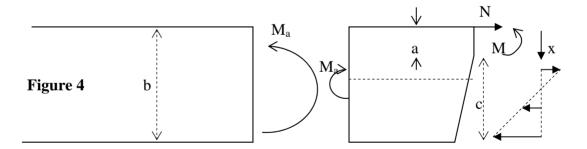
The moment per unit circumference acting on the uncracked section is  $M_a$ . We consider the Bueckner equivalent loading of the crack face, as shown above. This stress is  $\sigma(x) = \sigma_b(2x/b-1)$ , and the crack face lies at x = [a, b]. Integrating the net load on the crack face thus gives,
