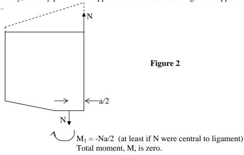
Hence, with carefully chosen positioning of the applied force, the rotation of the end of the plate can be made to be zero. This is the familiar "edge cracked plate, bending restrained"...
