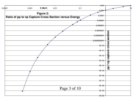
At ~0.1MeV, the proton-proton capture cross section is about 5 orders of magnitude smaller than the neutron-proton capture cross section. At ~1keV the difference is about 15 orders of magnitude. The latter is due largely to the Coulomb barrier. However, the small proton-proton capture cross-section compared with that of neutron-proton capture at ~0.1MeV is mostly due to the fact that the former involves identical particles.
