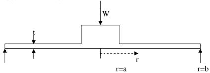
The shear load resultant at radius r is clearly  $F = \frac{W}{2\pi r}$ . (18)
