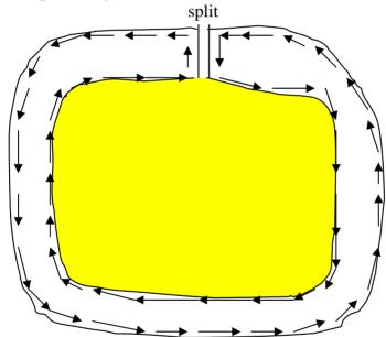
The major difference is the reversal of the direction of the shears caused by the new free surface at the split. This means that the area within the "onion skin" does *not* include the area within the 'bore' - shown shaded yellow above – whereas previously it did.
