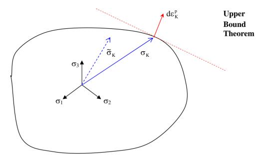
The differences are that, (a)the stresses with and without the tilda have swapped places, and, (b)the plastic strain increment is postulated rather than the true one. The stress without the tilda is defined as the stress corresponding to the postulated plastic strain increment. The stress with the tilda is the true collapse stress.
