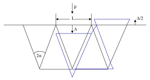
The blue lines show the displaced triangles – on one side only – due to a downwards displacement of the indenter by  $\Delta$ . (Apologies for the distortions – either my skill with WORD is poor, or the software is not up to the job).
